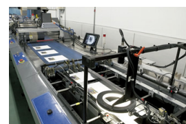
Our Attacher System, which automatically attaches and packs thin samples.
